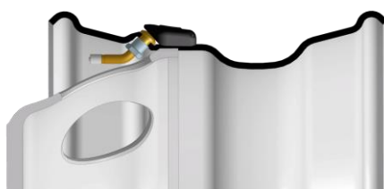
DCW-G2 – old generation Wheel with external valve with hump
