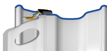
DCW-G3 – new generation Wheel with external valve without hump
